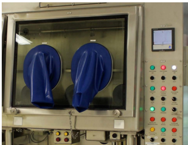
FIGURE 29.6 Isolator used in aseptic operation (Courtesy Janssen Pharmaceutica, Belgium)
