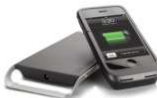
Fig. 16 Fulton Innovations' eCoupled Wireless inductive coupling charger [14]
