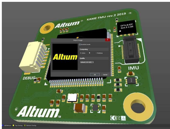
Logos and part numbers can be added to the silkscreen (overlay layers)
