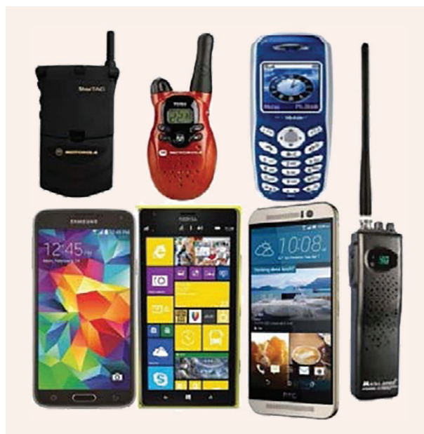
FIGURE 3. Examples of external and embedded/internal antennas used in commercial cellular and CB radios. (Source: [1].)
