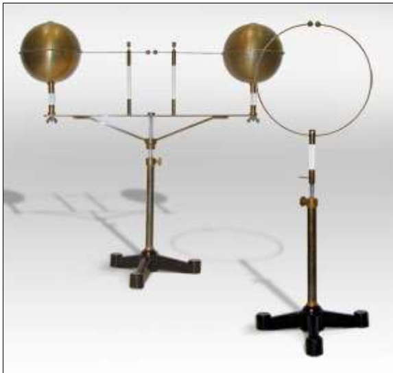
Early experimental Hertz radiator and resonator for creating and detecting Hertzian waves ~1890
