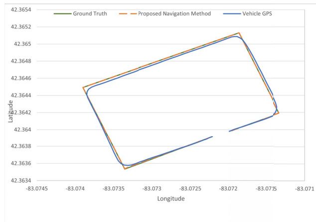
Fig. 9: Vehicle Location (Proposed Navigation System, Ground Truth and Vehicle GPS Comparison).
