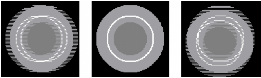
Example of Jagged / Banded Edges (Interlaced Video)
