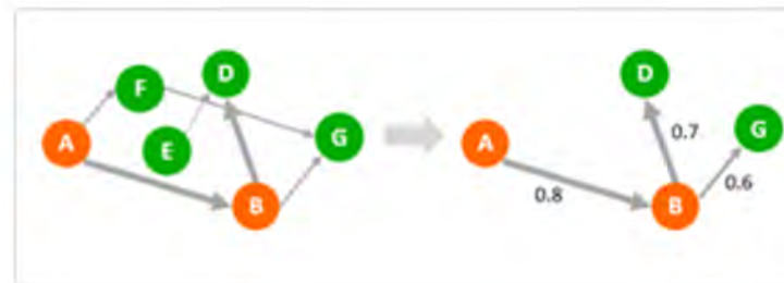
Figure 5: Expansion - aggregate weights and apply threshold
