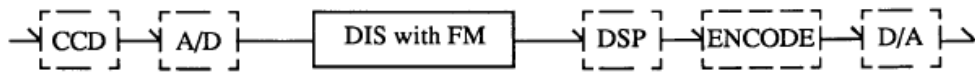
Figure 1. Block diagram of a digital video camera with a digital image stabilization (DIS) system and a field memory (FM).
