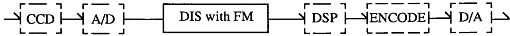
Figure 1. Block diagram of a digital video camera with a digital image stabilization (DIS) system and a field memory (FM).
