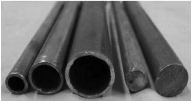
Figure 3. Indenters used in compression testing. Hollow indenters of 9.53, 12.70, and 19.10 mm diameter and solid indenters of 9.53 and 12.70 mm diameters are shown.
