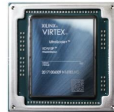
AMD VU13P FPGA: lidless package is used by BittWare's Viper thermal management for enhanced cooling performance
