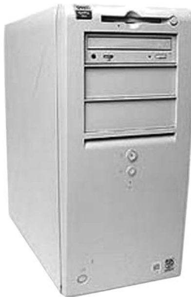
Figure 21.1 Typical tower case arrangement
