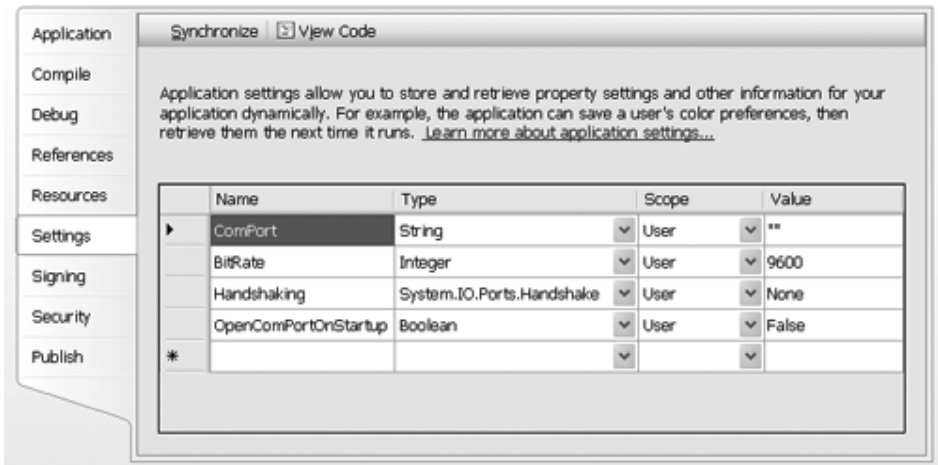
Figure 9-1: In Visual Studio's Project > Properties windows, the Settings pane enables defining application-specific values to be saved with an application.
