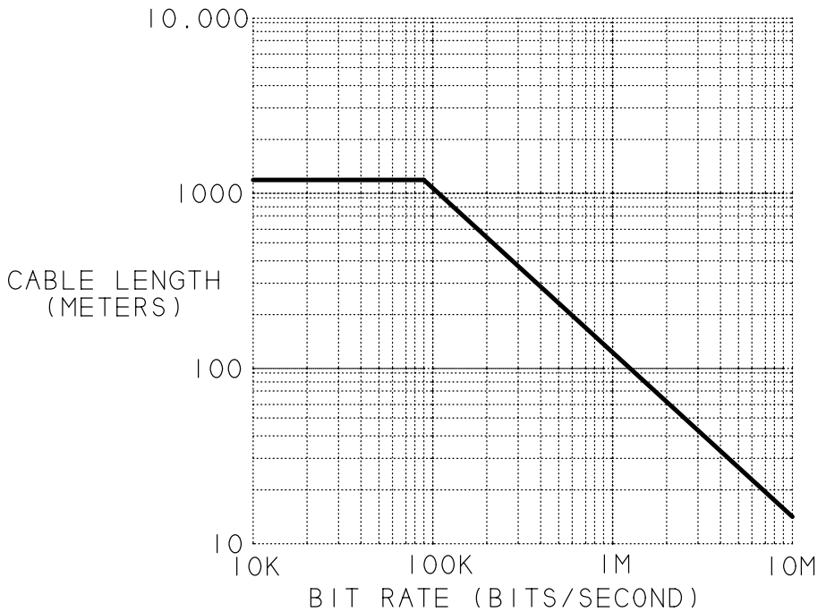
Figure 6-4: RS-485 supports transmissions up to 10 Mbps, but the higher bit rates require shorter cables.
