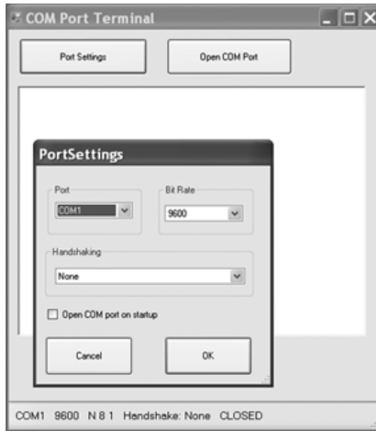
Figure 10-1: In this application, clicking the Port Settings button brings up a window that enables selecting a port and setting port parameters.
