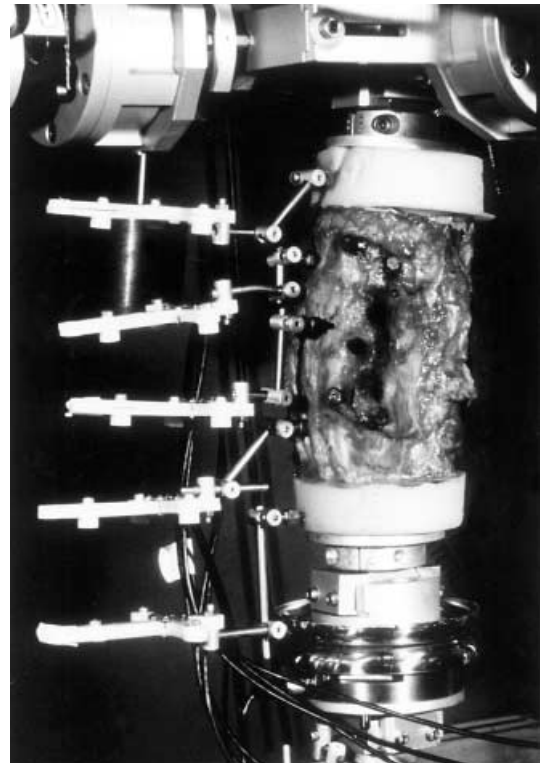
Fig. 3 Biomechanical investigation on an explanted specimen (patient 2, T12-L4) using a universal spine tester. L2 corpectomy and implantation of the PU-C vertebral replacement had been performed 15 months previously. Resulting three-dimensional displacements were measured between all adjacent segments with an ultrasound motion measurement system
