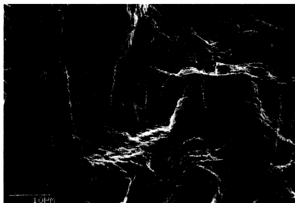
Fig. 5: Stainless steel fracture surface with horizontally oriented fatigue striations superimposed on longitudinally oriented slip systems characteristic of cubic face centred metals.
