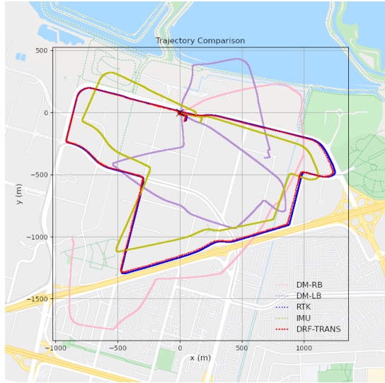
Fig. 11. Ground truth and model predicted trajectories over Sunnyvale Loop. The trajectory predicted by DRF-TRANS almost overlapped with the ground truth, and much more accurate than that of DM-RB or DM-LB
