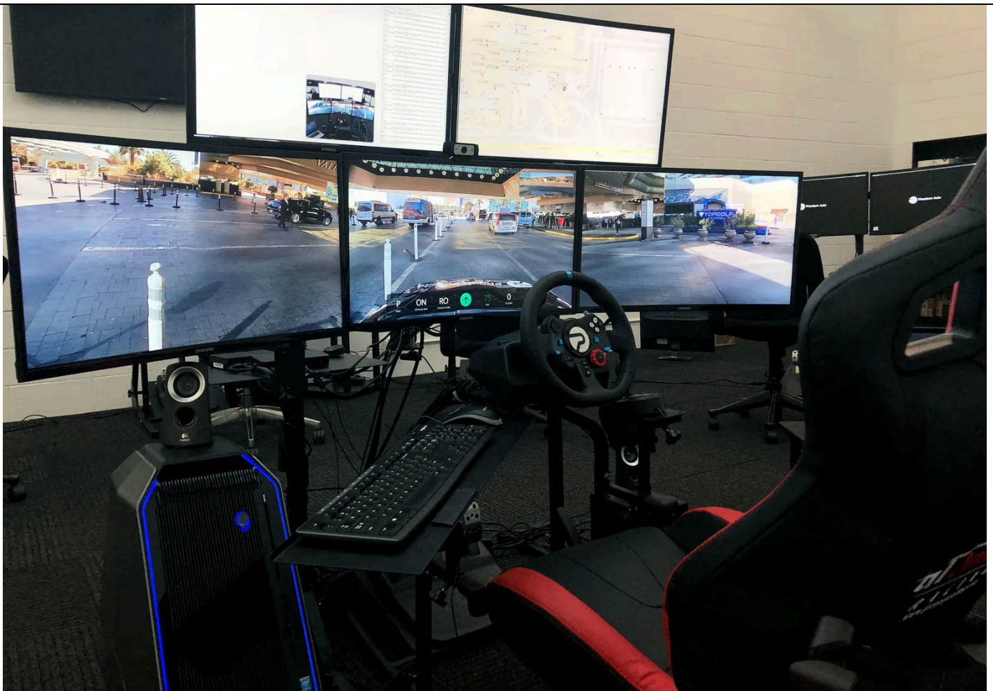
If a car gets in trouble, a human can use the car's cameras and microphone to grok what's going on. PHANTOM AUTO ADVERTISEMENT
