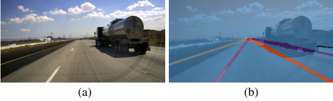
Fig. 7. Result of the segmentation model. (a) An input image. (b) Segmentation model output where each color represents each semantic lane boundary instance.
