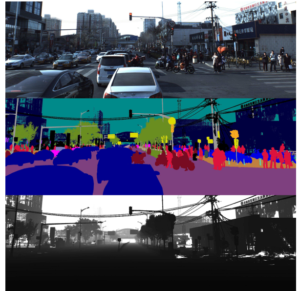
Figure 1. An example of color image ( top ), 2D semantic label ( middle ), and depth map for the static background ( bottom ).
