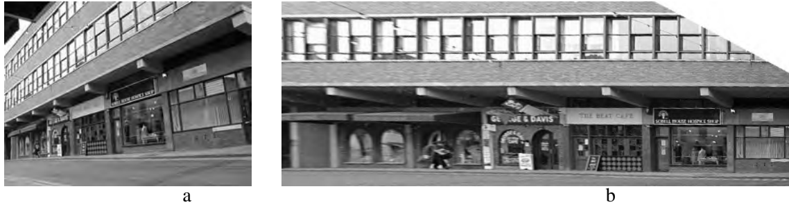
Fig. 8.25. Plane rectification via partial internal parameters (a) Original image. (b) Rectification assuming the camera has square pixels and principal point at the centre of the image. The focal length is computed from the single orthogonal vanishing point pair. The aspect ratio of a window in the rectified image differs from the ground truth value by 3.7%. Note that the two parallel planes, the upper building facade and the lower shopfront, are both mapped to fronto-parallel planes.
