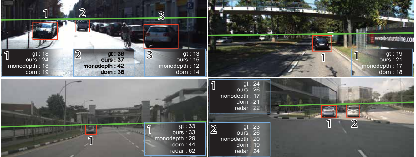
Figure 6. Sample results on Kitti [12] (top) and nuScenes [3] (bottom). Displayed numbers are the distances in meters. Vehicles are numbered for clarity.
