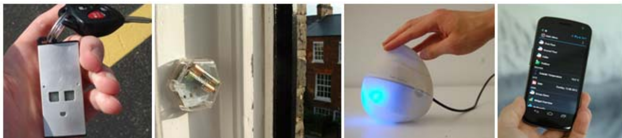
Figure 9. IOT Home Automation and Environment Monitoring Innovations: Sensordrone, Flexibity Internet Sensors, Air Quality Egg, and openHAB on Android.
