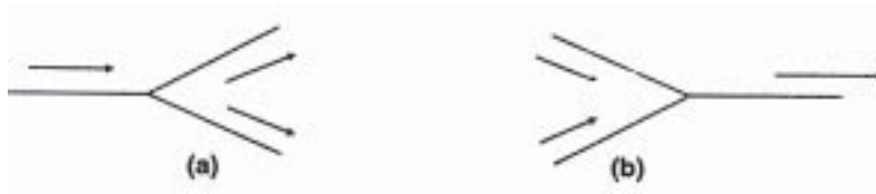
Figure 5. (a) Three port coupler as a splitter. (b) Three port coupler as a combiner.
