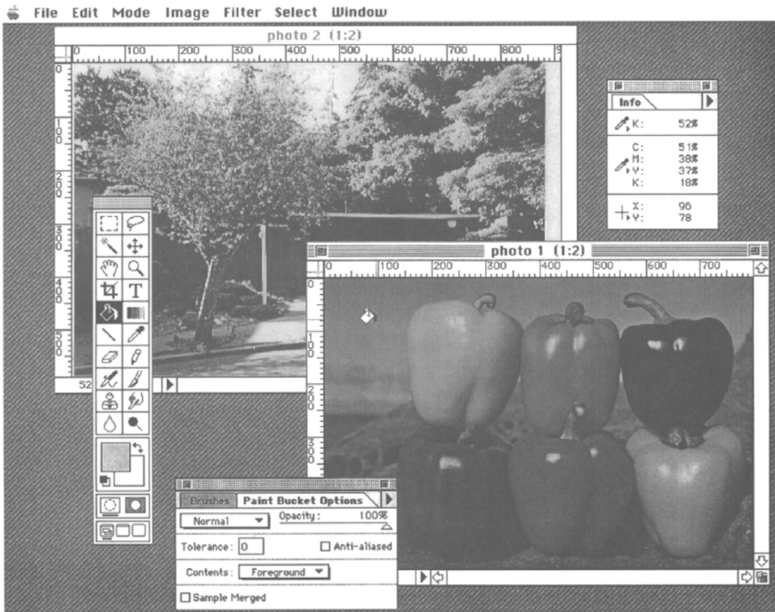
Figure 1. Typical applications operating in the Apple Macintosh® GUI. Single or multiple windows can be moved and resized. Toolboxes and dialogue boxes can also be placed where needed. Pointer signs automatically change as required by the state of the system.
