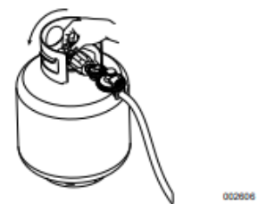
Figure 2-17. Turn LPG Tank Valve On
