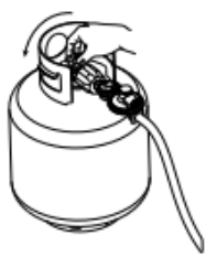
Figure 2-17. Turn LPG Tank Valve On
