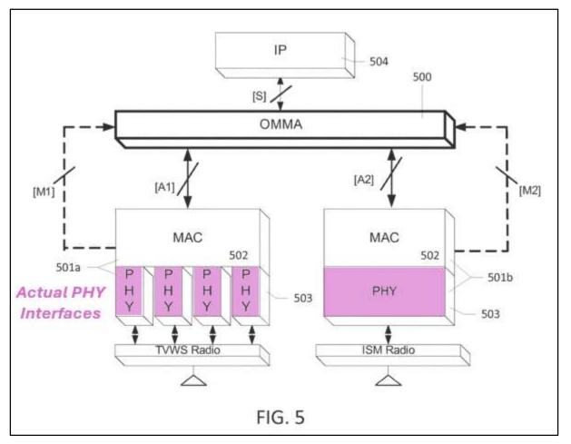
(e) 1[d]: first and second wireless transceivers respectively associated with the first and second actual PHY interfaces, wherein the first and second wireless transceivers (i) are suitable for use in a wireless local area network, (ii) respectively have first and second bandwidth availabilities up to first and second actual bandwidths, and (iii) are adapted to respectively emit radio waves in first and second different bands of frequencies; and
