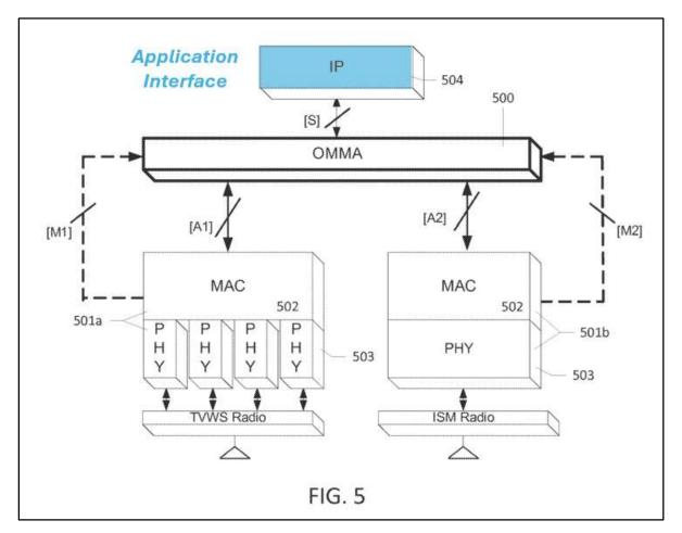
*"a processing interface configured to, during use of the wireless networking device, interact with an application":* Chincholi further discloses that its "application interface" is connected to and interacts with a "processing interface." (EX1002 ¶84.) Chincholi's *processing interface* is referred an "*Opportunistic Multiple-Medium Access Control (MAC) Aggregation (OMMA) layer*." (EX1005
