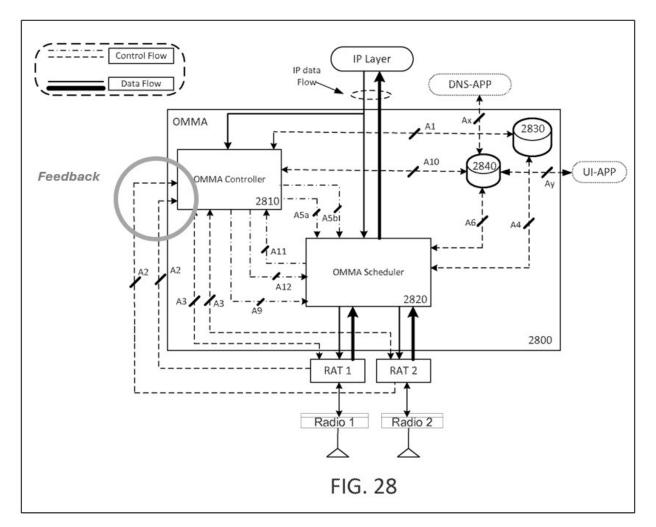
The Feedback Device Classifier module (i.e. resource monitoring interface) collects information directly from each of the first and second transceiver resources/requirements over the "A2" interfaces in the diagram above so that this information may be fed back to the OMMA Scheduler. (EX1002 ¶133.) Chincholi's Figure 5 shows that the RAT-side of the "A2" interface is the *actual MAC interfaces*:
