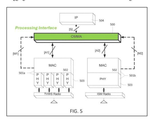
The IP layer is connected to the OMMA layer and provides IP packets that the OMMA layer processes. (EX1005  $\P[0138]$ ); (EX1002  $\P85$ .) The OMMA "may allow for enhanced throughput and reduced latency for a single IP flow." (EX1005  $\P[0120]$ .) The OMMA layer is therefore a processing layer, which processes IP packets and provides an *interface* between the IP layer and actual MAC layers, *i.e.*, a *processing interface*.
