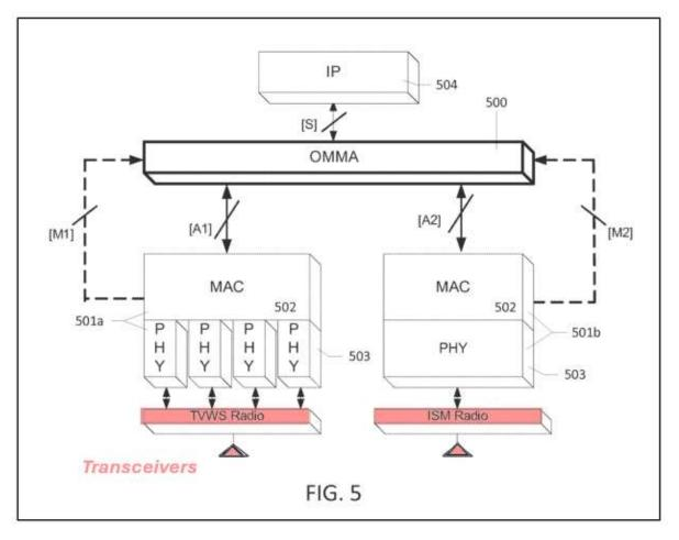
A POSITA would have understood that a "transceiver" is a physical device that can both transmit and receive information. (EX1002 ¶91.) Thus, each of Chincholi's disclosed "antenna/RF front-end pairs" are a transceiver because they operate on wireless protocols that both transmit and receive data, such as IEEE802.11, IEEE802.11ac, IEEE802.11af, LTE, WCDMA, etc. (EX1005 ¶[0134].)
