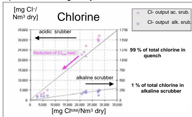
**Total intermediate Cl<sub>2</sub> in boiler flue gas:**
