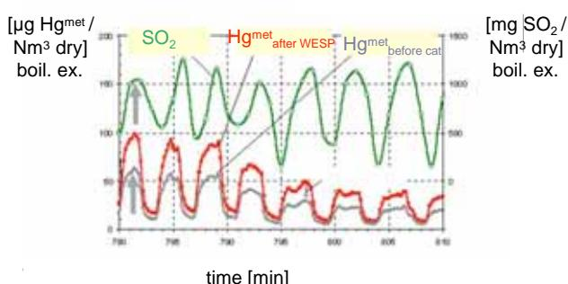
Cl<sub>2</sub> resuppression by SO<sub>2</sub> in boiler --> less Hg<sup>ox</sup> at boiler exit
