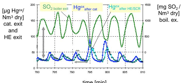
less residual SO<sub>2</sub> --> less Cl<sub>2</sub> in SCR --> less Hg-oxidation in SCR
