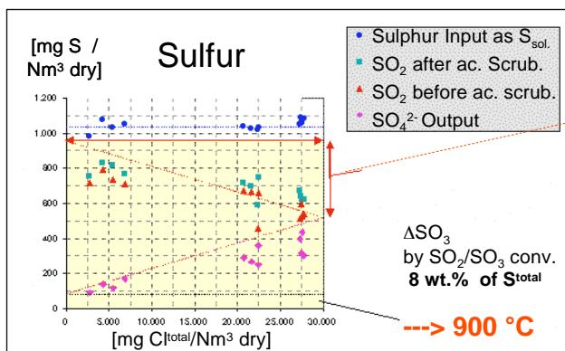
$$\begin{aligned}\Delta S &= 400 \text{ mg S/Nm}^3 \text{ dry} \\ &= 12.5 \text{ mmol S/Nm}^3 \text{ dry} \\ \Delta Cl_2 &= 12.5 \text{ mmol Cl}_2/\text{Nm}^3 \text{ dry} \\ &= 886 \text{ mg Cl}_2/\text{Nm}^3 \text{ dry}\end{aligned}$$
