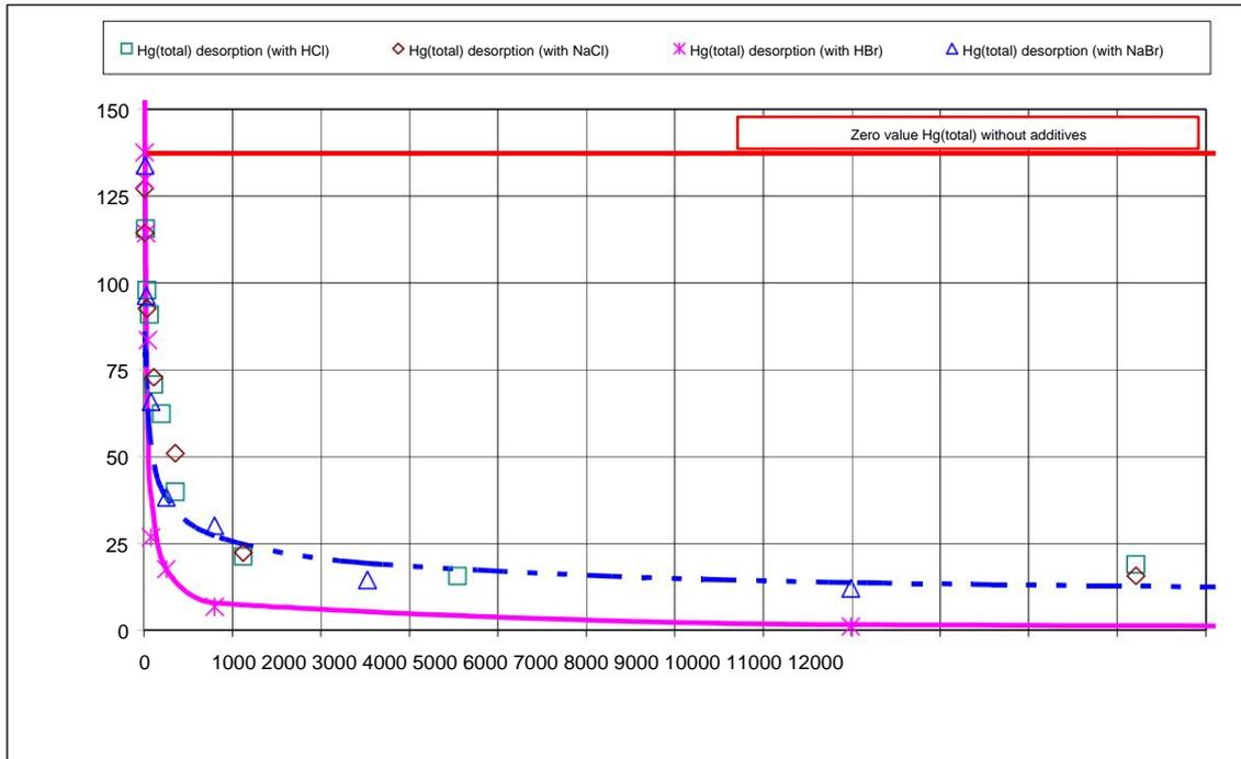
It was thus shown, as already well known from the complexation of HgCl<sub>2</sub> by chloride, that by increasing the halide concentration (and thus the conductivity in the scrubber) a almost complete retention of the oxidized mercury in the acidic wash solution
