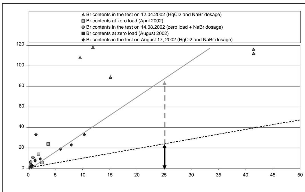
The abscissa and thus also the dashed diagonal of the image describe the calculated Bromine content corresponding to the Hg content (bromine as adsorbed HgBr<sub>2</sub>); assuming Adsorption of bromine only in the form of mercury bromide (HgBr<sub>2</sub>) should reduce the Hg and Bromine contents are in a stoichiometric ratio (dashed diagonal).
