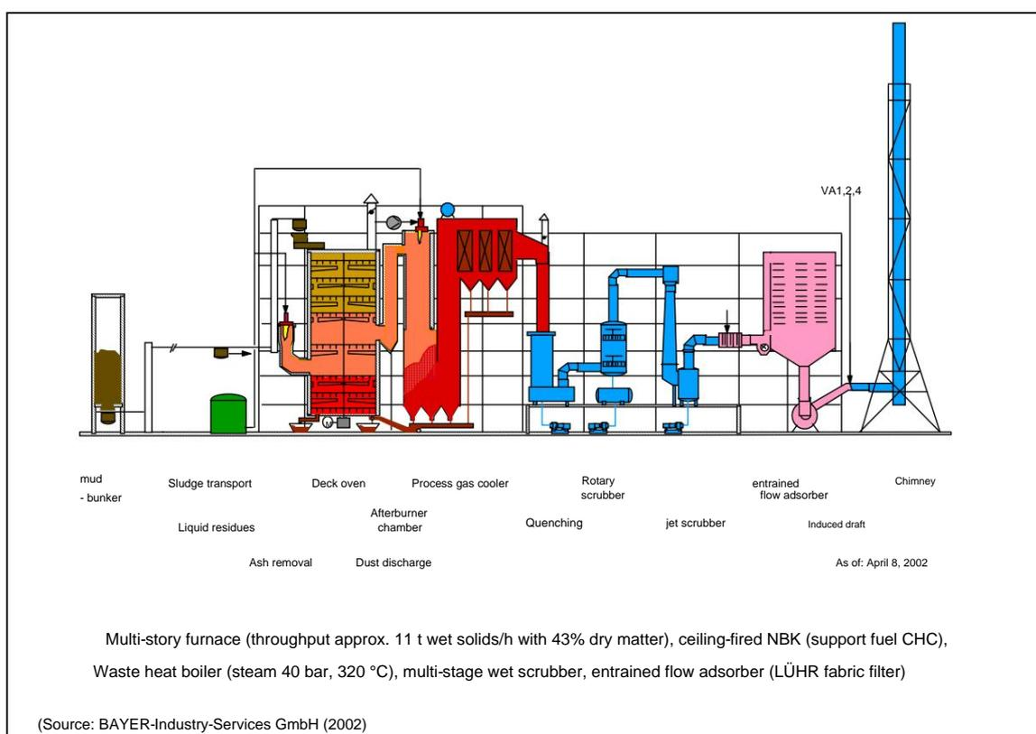
During normal plant operation (CHC co-combustion), mercury oxidation is always ensured due to the high Cl load in the boiler flue gas, and thus, wet mercury separation in the multi-stage flue gas scrubber (RGW) was not a problem anyway.
