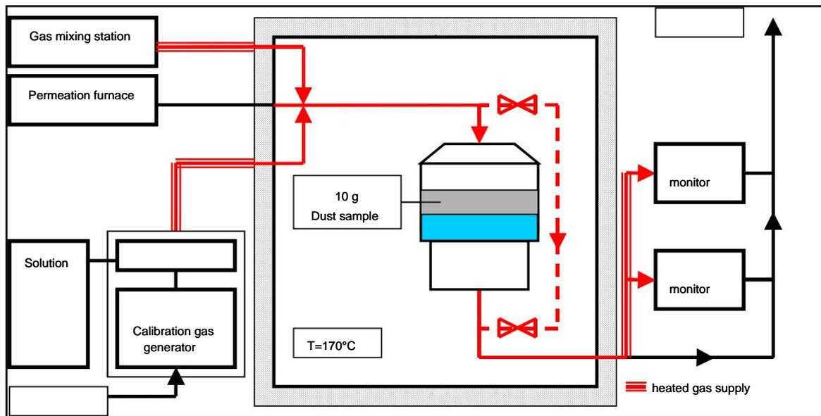
To generate defined Hg model gas concentrations and Hg species fractions, a Hovacal liquid evaporator (HgCl<sub>2</sub> as primary Hg ion) and an MKal-Permeation evaporator (Hgmet). Acidic components (such as HCl and HBr) and water vapor are also supplied as aqueous solutions via the Hovacal evaporator. Additional model gas components (e.g., SO<sub>2</sub>) are provided via a gas mixing station.
