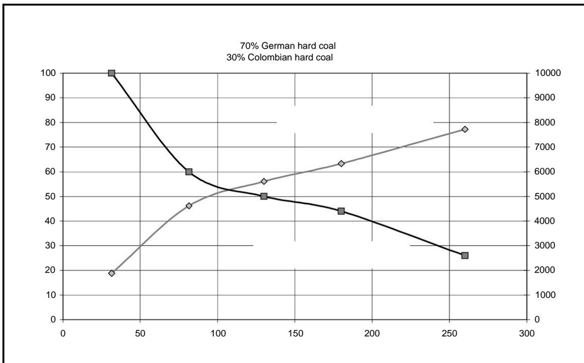
In the lower grain size range, as can be seen to read an increase in Hg-content with the C content; in the upper grain size range, however, the The question arises as to why this might be the case, since it is well known that "Carbon" leads to increased mercury adsorption compared to "quicklime" cf. e.g. Hocquel.
