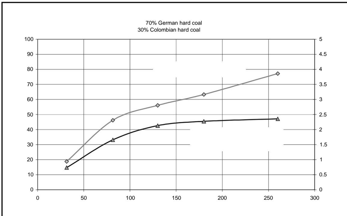
Common sorbent mixtures with PAC, HOK or carbon black additives have a different larger accessible internal surface, namely the "BET-Surface". If one applies the models described above to such C-based sorbent mixtures, it is not surprising that these in connection with "bromine" have a considerable Hg adsorption capacity, see Nelson /18/, /19/ on Hg-Adsorption on externally brominated sorbent mixtures with such additives (activated carbon, carbon black).
