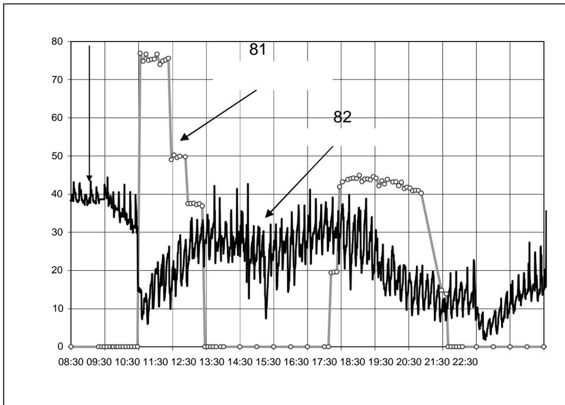
With the start of the addition of bromine into the SKK combustion chamber (in the form of aqueous NaBr-solution) at 10:30 a.m., the Hgmet/Hgges species content drops abruptly below 10 wt.%. A similar, albeit delayed, occurs again after 4:00 p.m. with renewed bromine
