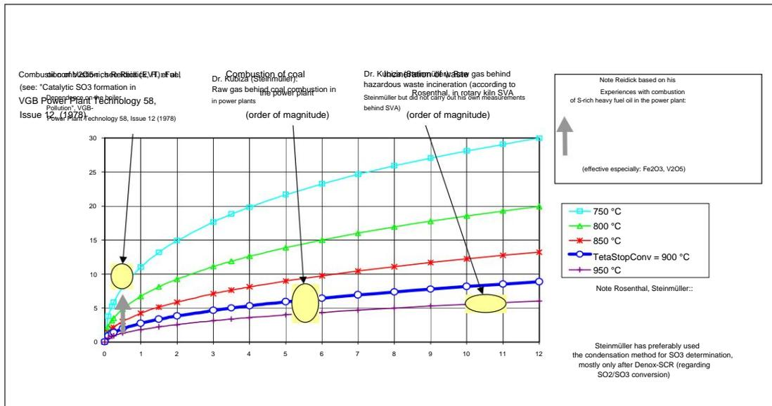
The SO<sub>2</sub>/SO<sub>3</sub> conversion by the flue gas oxygen is possibly catalytically mobilized by metal oxides in the flue dust such as iron oxide and vanadium pentoxide down to lower temperatures. an interesting operational example of this was provided by power plant investigations into Combustion of vanadium-rich heating oil, see Reidick
