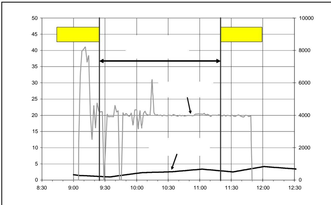
This exceptional experiment with discontinuous Hg addition was carried out under a (from the SVA perspective) only medium bromine load, namely a Br<sub>2</sub> content in the boiler flue gas of approximately 4,000 mg/Nm<sup>3</sup> d., and a residual SO<sub>2</sub> content at the boiler end of 5,000 – 6,500
