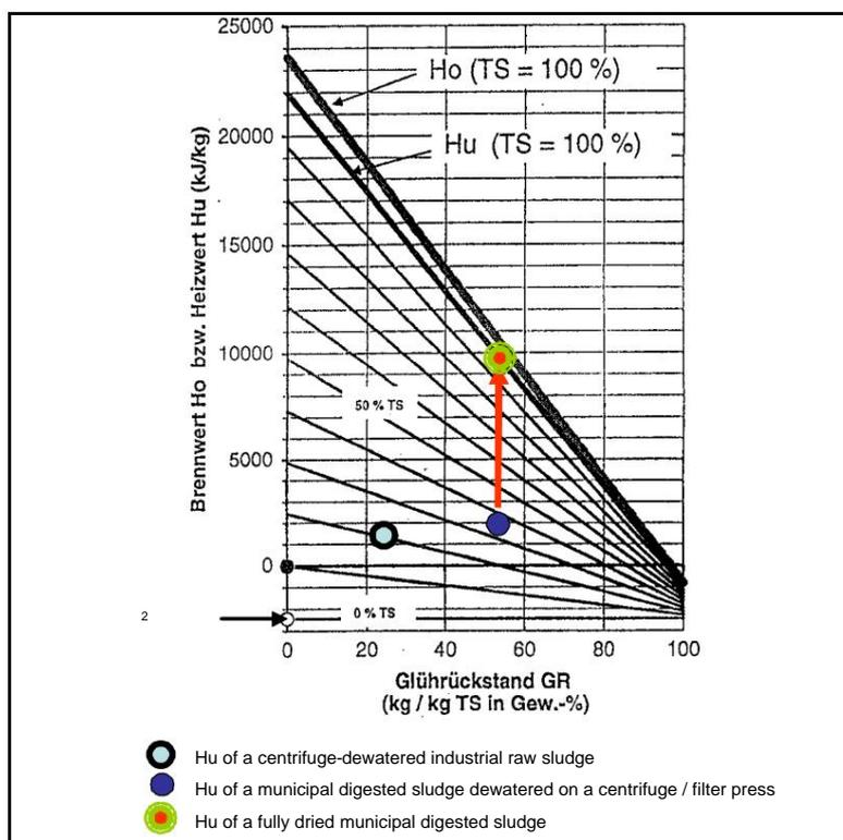
For various reasons, usually only a small proportion of fuel  $\ll 10\%$  of the thermal output of a power plant (calculated with the calorific value  $H_u$  of the dry substance) replaced by wet sewage sludge, although the 17th BImSchV allows up to 25% without the fuel plant as a whole into a waste incineration plant under the licensing law.
