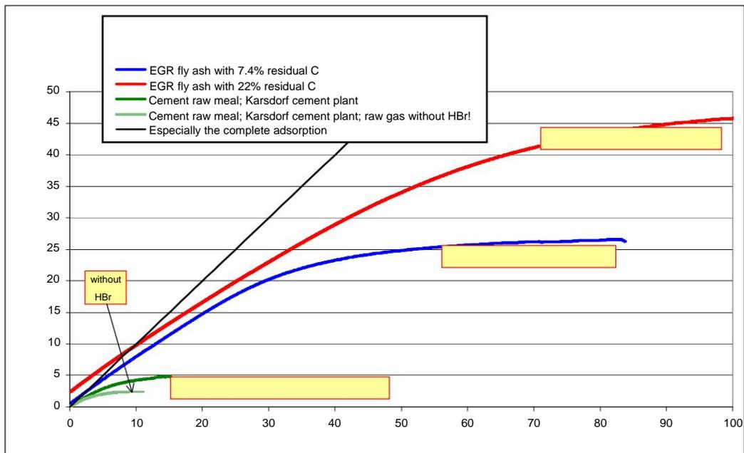
The cement raw meal examined from the Karsdorf cement plant is a thermally unstressed, residual C-free raw meal with 76.8 wt.% calcium carbonate (CaCO<sub>3</sub>) as Main component. The raw meal had an average grain size of 88 μm, cf.
