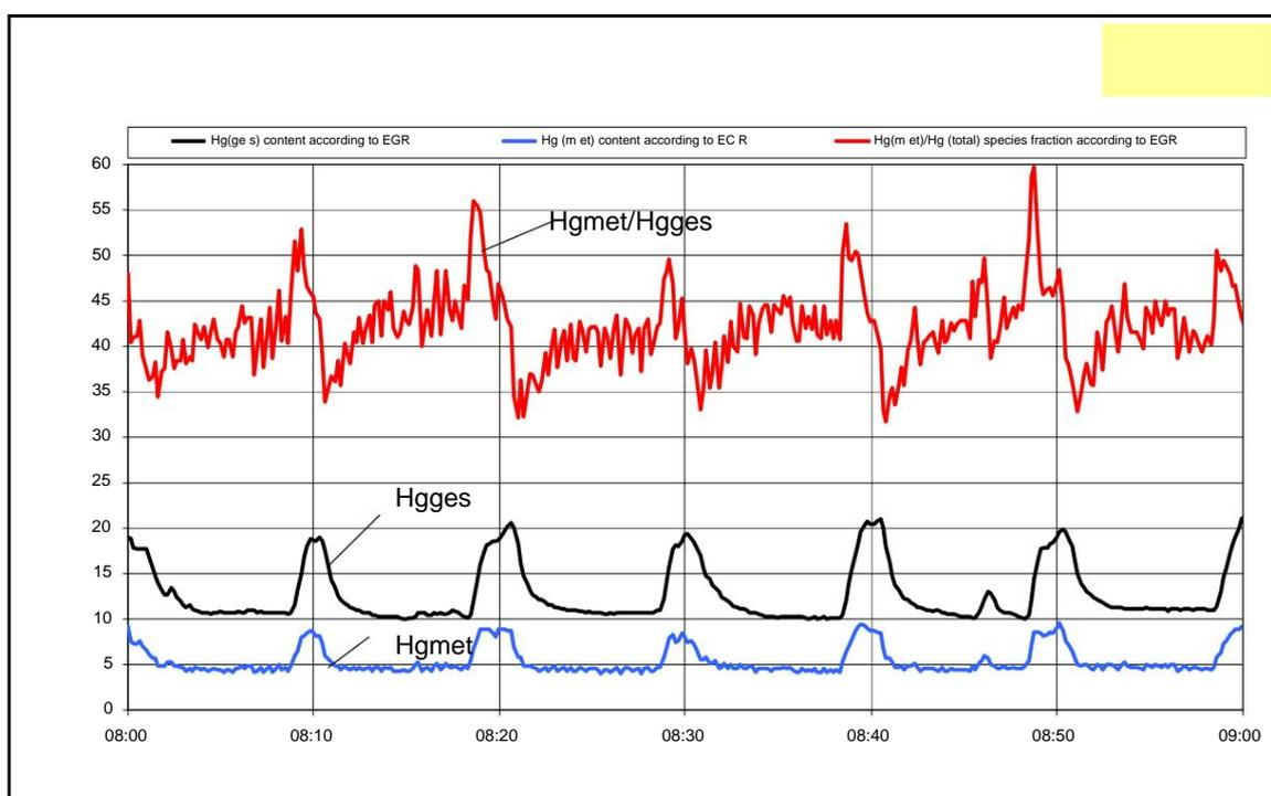
It is possible that there will be an increase in the dedusted clean gas up to the higher concentration level before EGR, which is likely to be above the coal-related base level (approx. 25  $\mu\text{g Hgges}/\text{Nm}^3$  tr. in April 2002, approx. 12  $\mu\text{g Hgges}/\text{Nm}^3$  tr. in August 2002) due to the dust recirculation (circulation between the SKK combustion chamber and EGR ).
