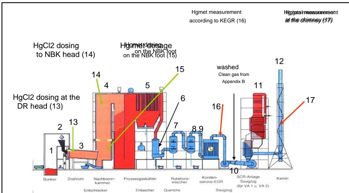
The illustration shows the rotary kiln SVA A with its bunker 1 for solid waste, the crane grab 2 as well as other feed devices for liquid waste and container waste (barrel elevator), the rotary kiln 3, the afterburner chamber 4, the waste heat boiler 5, the strongly acid quench 6, the acidic rotary atomizer washer 7, the weakly alkaline rotary atomizer
