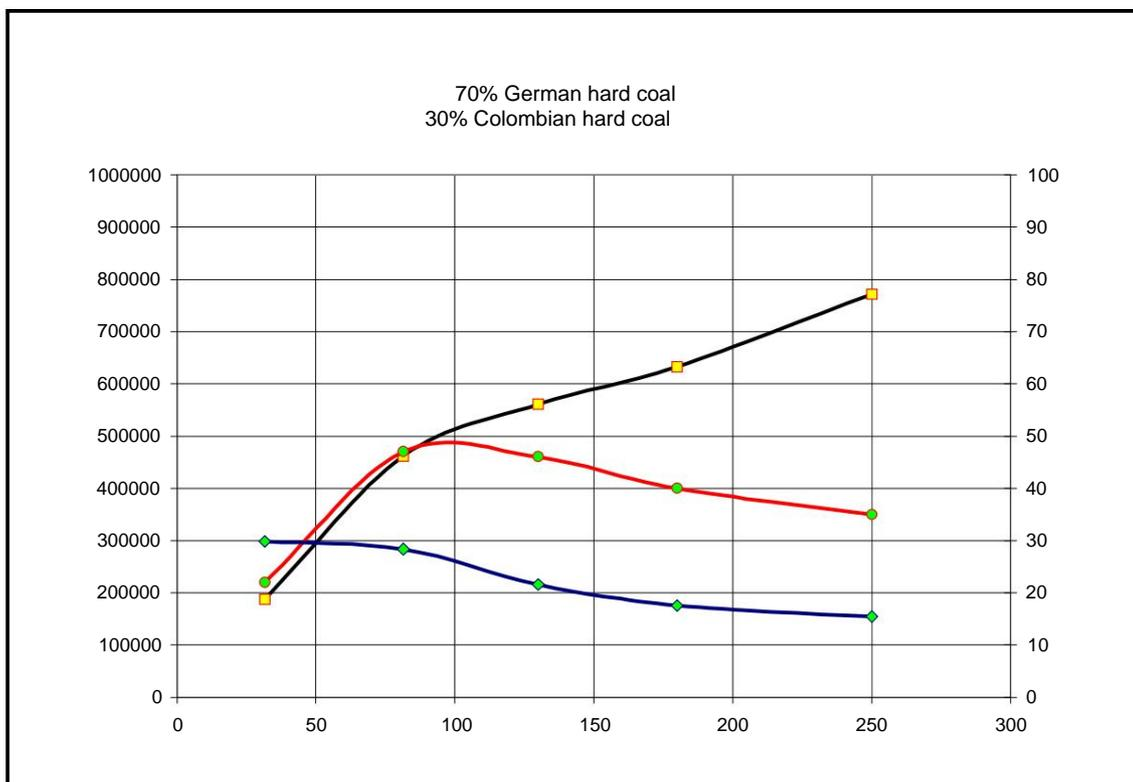
In Finally, the residual C content and the Hg loading of the calculated outer C-grain surface. This Hg loading increases with increasing Grain size to a "saturation value" of approx. 2.5 mg Hg/m<sup>2</sup>.
