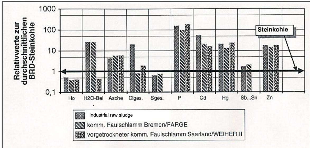
A particular problem is the relatively high mercury content of sewage sludge compared to coal (normally 1 - 2 mg/kg TS, occasionally higher), whether wet or dried, because Hg remains in the dry substance during gentle drying, cf.
