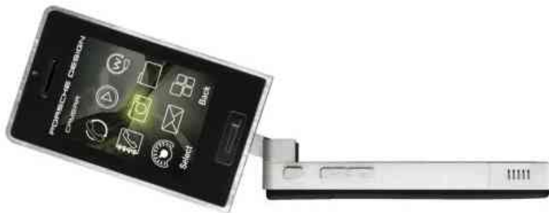
Figure 4: Mobile handset (the Porsche P'9521) equipped with fingerprint sensor (at bottom of screen). Source: Atrua Technologies.
