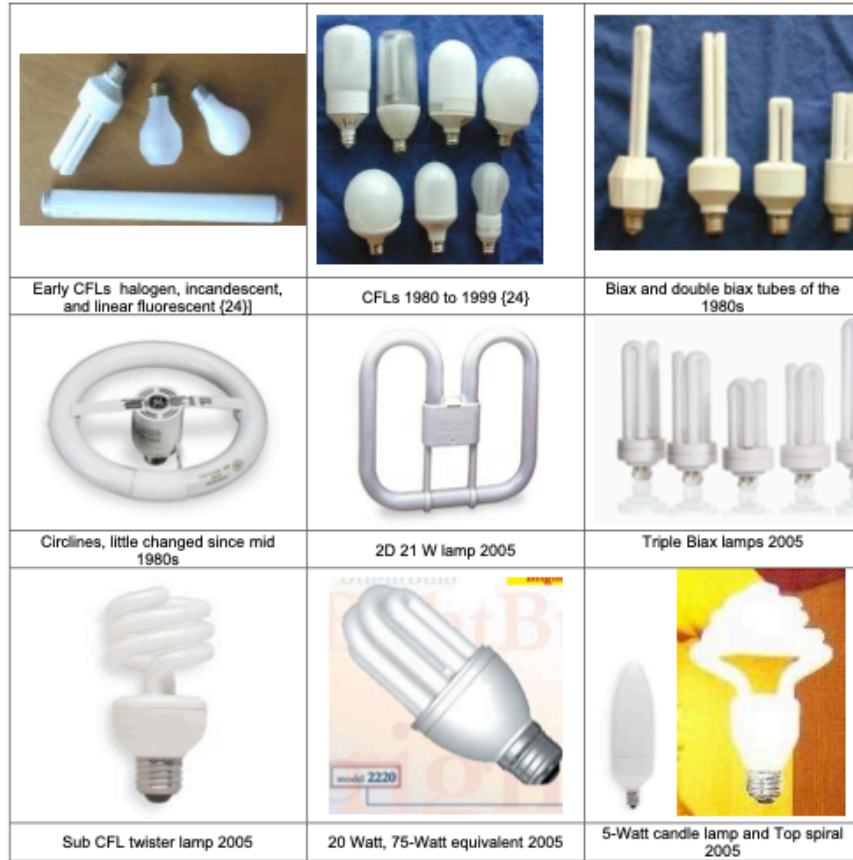
Figure 1.1. Evolution of Compact Fluorescent Lamp Designs. CFLs have come in a variety of shapes and sizes, but the overall trend has been downsizing from the early 2-foot-long U-tubes of the 1970s (which were basically a 4-ft long, 1.5-inch-diameter T-12 bent in half) to the T6 0.5-in.-diameter U-tube (6-in. lamp length plus ballast) of the mid 1980s, to the triple tube or triple biax lamps (4.9 in. lamp, 6 in. with ballast) and double U tube (3-in. lamp length plus ballast) designs of the mid 1990s, to the 4.0-in. twister lamps that first appeared in 1995.
