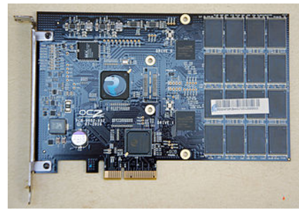
An OCZ RevoDrive SSD, a full-height ×4 PCI Express card
