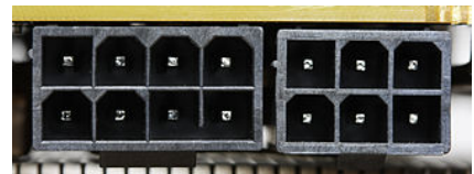
8-pin (left) and 6-pin (right) power connectors used on PCI Express cards
