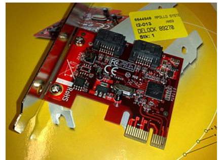
A Marvell-based SATA 3.0 controller, as a PCI Express ×1 card
