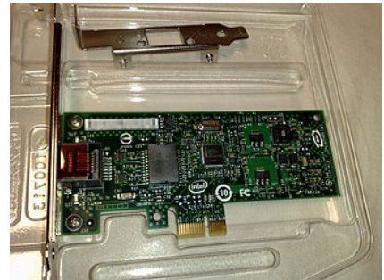
Intel 82574L Gigabit Ethernet NIC, a PCI Express ×1 card
