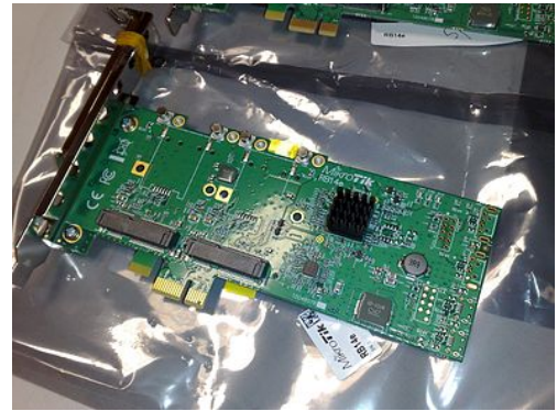
A PCI Express ×1 card containing a PCI Express switch (covered by a small heat sink), which creates multiple endpoints out of one endpoint and allows it to be shared by multiple devices
