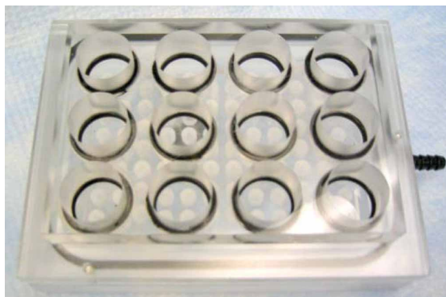
Figure 11 | Picture of the infectious center assay apparatus. Twelve wells are used to vacuum samples onto a HyBond XL nylon membrane (Amersham Biosciences) placed between the top plate and middle plate.
