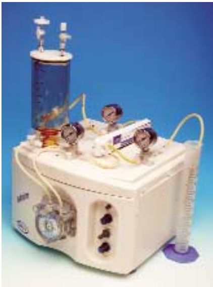
A Minimate TFF Capsule device for development and processing applications using small sample volumes. Samples can be concentrated down to about 5 mL and diafiltered. PALL CORPORATION (WWW.PALL.COM)
