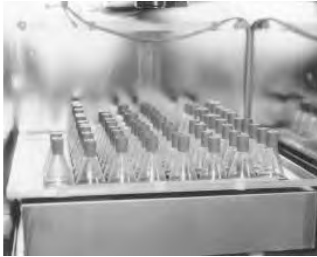
Fig. 2. View inside an incubator containing a gyratory shaker. The culture flasks (here 50-mL Erlenmeyer flasks with gas-permeable caps) are kept in ranges of 10 (max load 100 flasks). Attached to the shaker platform is a thermometer to show the local temperature (kept between 36.5 and 37°C).
