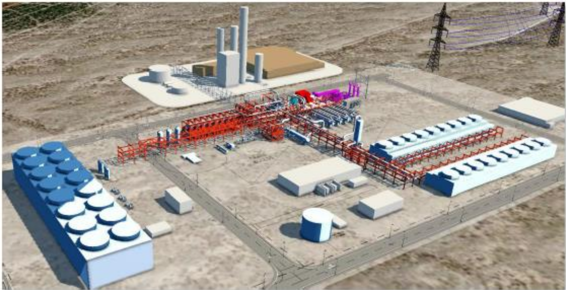
Figure 2: NET Power nominal 300MWe Commercial Plant Concept
