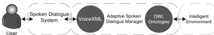
Fig. 1.1 The underlying idea of a layered ASDM architecture
