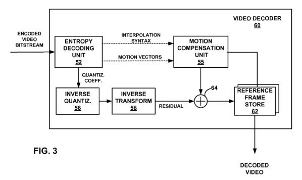
On the decoding side, motion compensation unit 55 may receive a syntax element from entropy decoding unit 52 identifying an interpolation filter among several available. *Id.* Motion compensation unit 55 generates prediction data by interpolating pixel values of the reference video data using the interpolation filter identified by the syntax element. *Id.*
