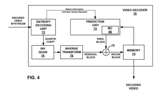
In the block diagram, video decoder 70 includes entropy decoding unit 72, prediction unit 75, inverse quantization unit 76, inverse transform unit 78, memory 74 and adder 79. *Id.* ¶ 83. Prediction unit 75 includes motion compensation (MC) unit 88 and spatial prediction components, not shown. *Id.*
