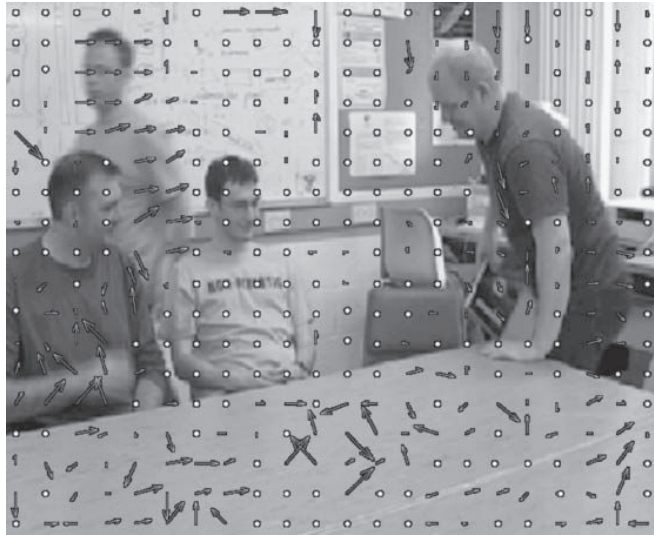
Figure 3.56 16 \times 16 motion vectors superimposed on frame
