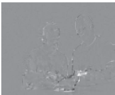
Figure 3.14 Residual : 8 \times 8 block size
