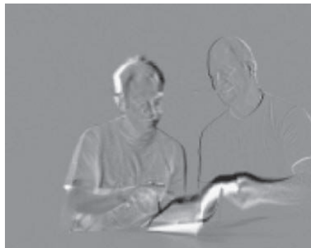
Figure 3.12 Residual : no motion compensation
