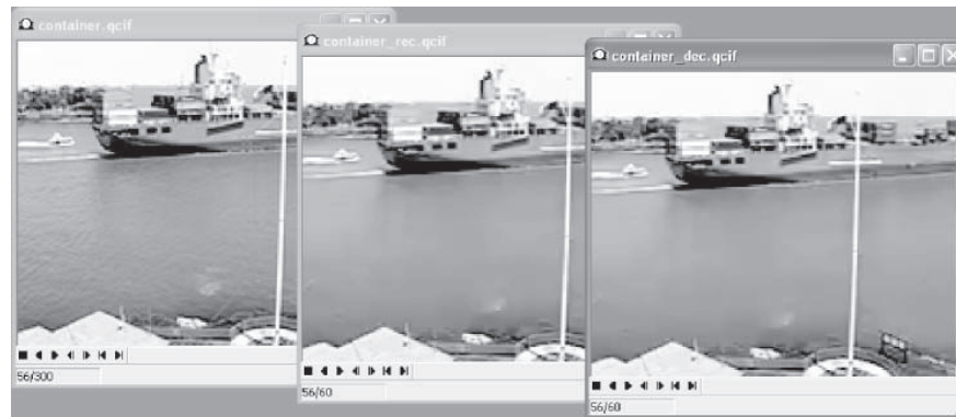
Figure 9.5 Original, reconstructed and decoded frames, container.qcif, QP=32
