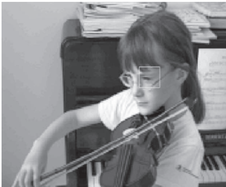
Figure 6.6 QCIF frame with highlighted macroblock
