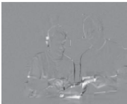
Figure 3.13 Residual : 16 \times 16 block size
