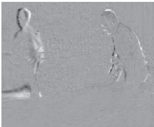
Figure 3.55 Residual F_n - F'_{n-1} : no motion compensation
