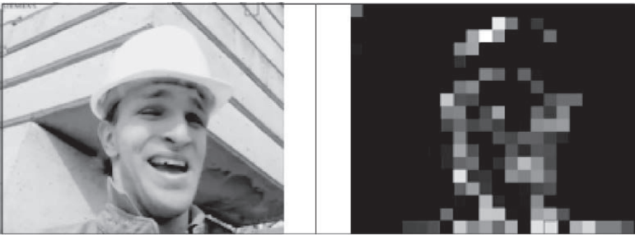
Figure 9.20 Frame from ‘Foreman’ sequence showing macroblock sizes
