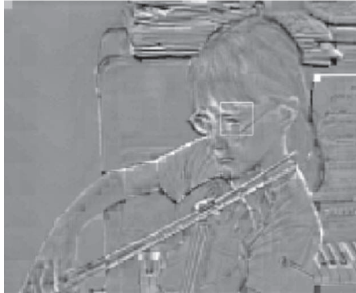
Figure 6.8 Residual after subtracting intra prediction
