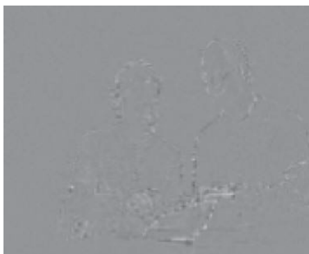
Figure 3.15 Residual : 4 \times 4 block size
