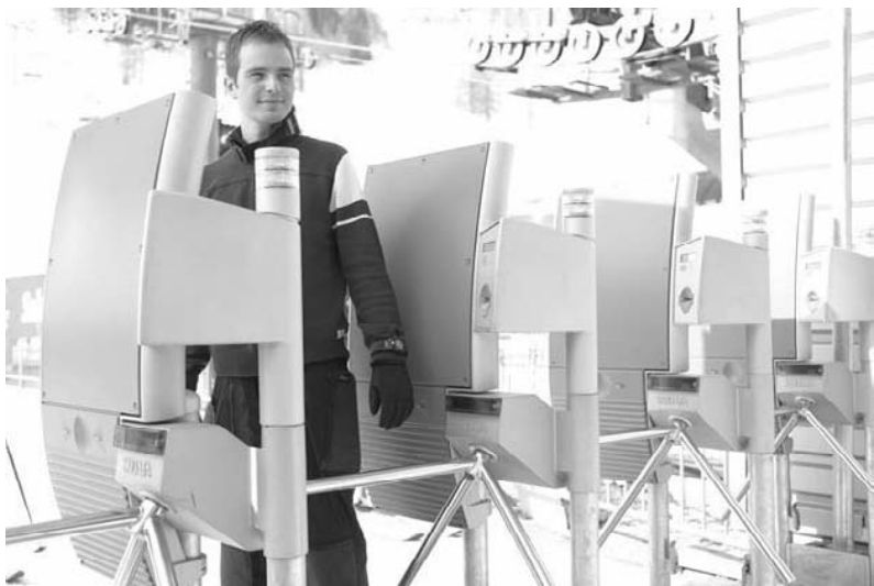
Figure 13.22 Contactless reader as access control and till device at a ski lift (reproduced by permission of LEGIC Identsystems AG, CH-Wetzikon)
