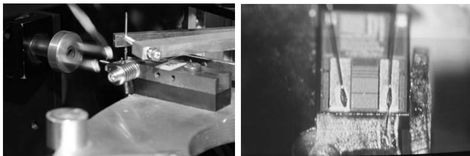
Figure 12.4 Left: the transponder coil is wound around the ferrite core. Right: contacting the coil to the chip (reproduced by permission of : AEG Identifikationssystem GmbH, RFID im Blick)
