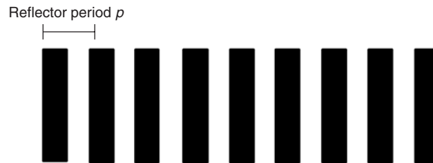
Figure 4.96 Geometry of a simple reflector for surface waves (reproduced by permission of Siemens AG, ZT KM, Munich)
