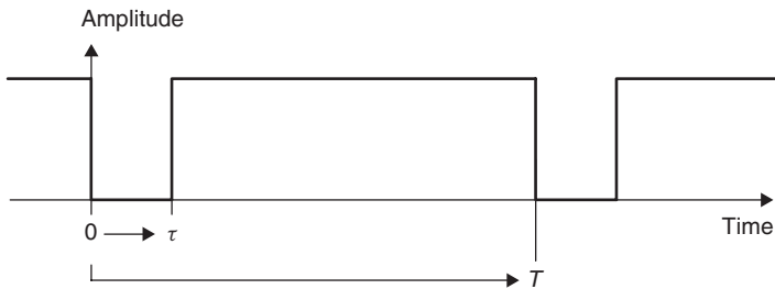
Figure 6.8 Representation of the period duration T and the bit duration \tau of a binary code signal
