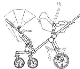
Reference drawing illustrating the status of usage of the present invention additionally installed with a storage basket + a safety seat + a cabin
