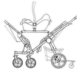
Reference drawing illustrating the status of usage of the present invention additionally installed with a storage basket + two cabins + a skate board + a safety seat
