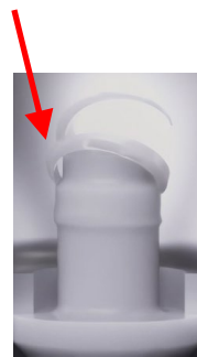
“Pin Capture” (pulled out of abutment)
