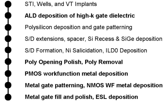
Fig.5 Transistor process flow highlighting differences from [6,7]
