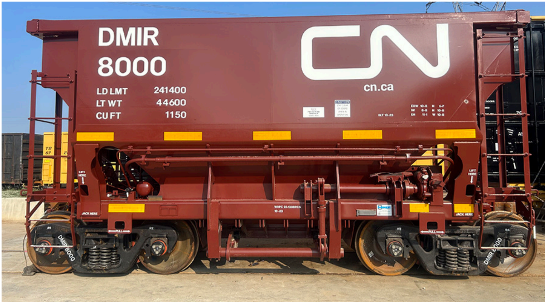
A specialized type of hopper car designed to haul heavy loads of iron ore, the new cars feature a small capacity due to increased load density. CN
