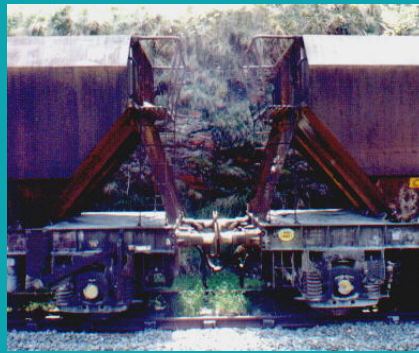
Above Left : Ends of the wagons showing how the handrails slope outwards and buffing details. Wagons have two brake pipes - one Yellow and one Red - only the Red pipe is connected as this is the train air pipe. Instanter couplings are fitted to all wagons.
