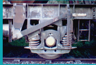
Above Right : This is the unit as fitted to the right-hand end of the wagon - these units are handed - the difference being the fact that the longer spring always faces the headstocks whilst the 'teeth' face inwards - the 'teeth' is the covering over the inner spring. The right hand unit on these wagons also has the hand-brake lever mounted in front a standard fitting - the levers are fitted at the opposing corners i.e. at right-end of wagon. All wagons have clasp brakes and plain disk wheelsets.
