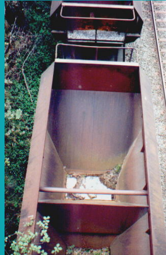
Above Right : A view directly inside one of the PGAs with debris atop of the hopper doors. Note the centre arch which divides the load into half for unloading purposes. A tubular crossbar strengthens the sides of the wagon.
