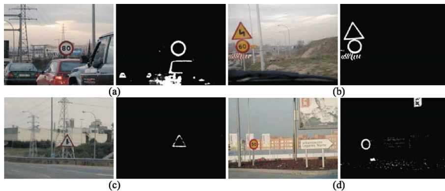
Fig. 3. Colour detection. (a, d) Other objects with the same colour presence; (b) union of two signs to form only one object; (c) some points of the sign are badly classified.
