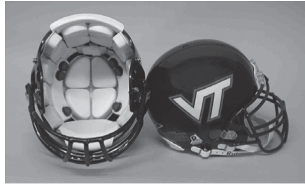
FIGURE 2. Virginia Tech helmet with the player unit installed.
