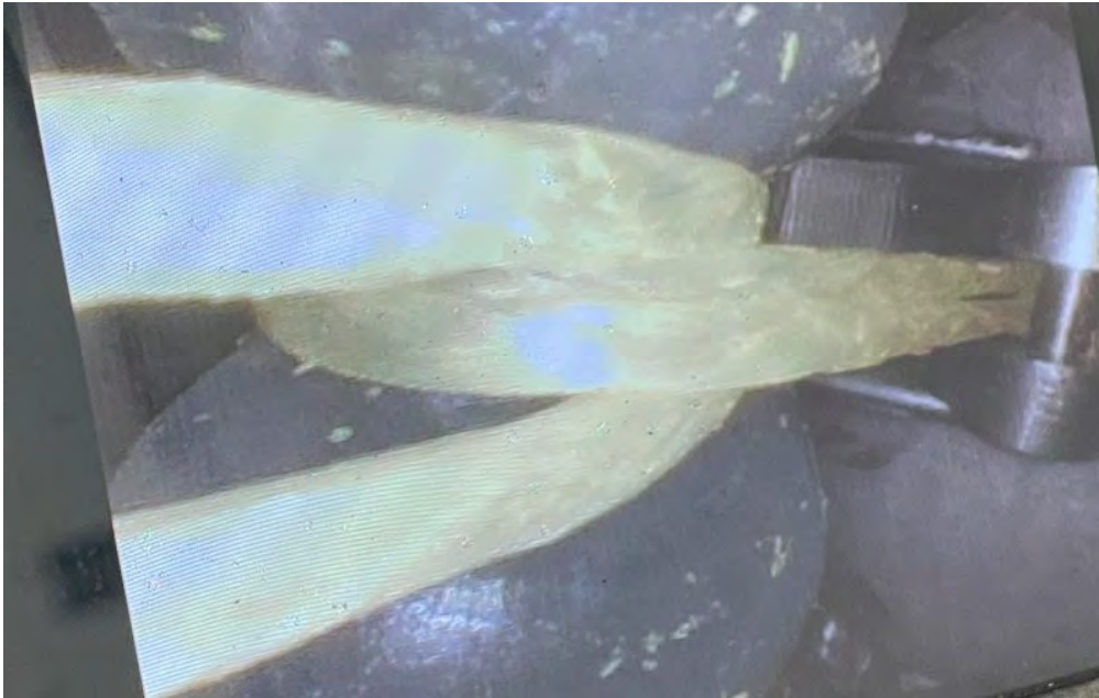
(Internal image of side view of elongate (tubular) member of the hemostasis valve with filaments encircling and constricting elongate member in the first (undepressed button) position.)
