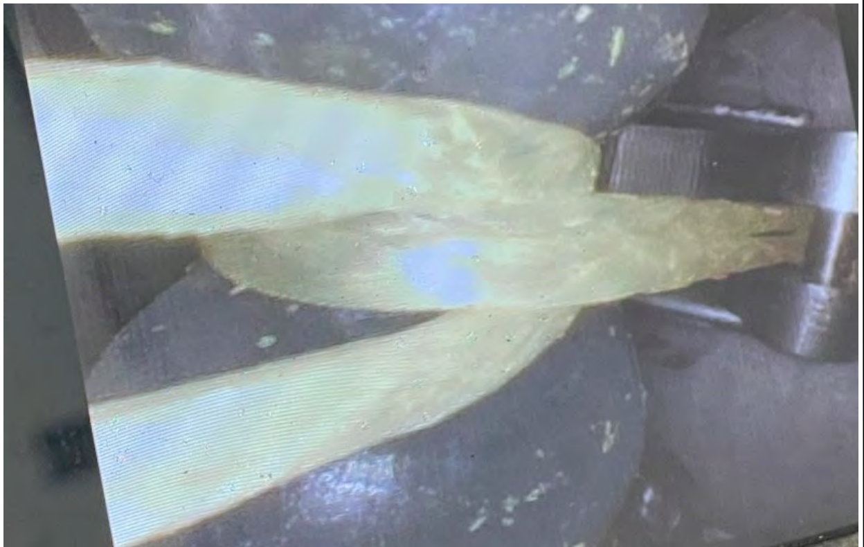
(Internal image of side view of elongate (tubular) member of the hemostasis valve with filaments encircling and constricting elongate member.)
