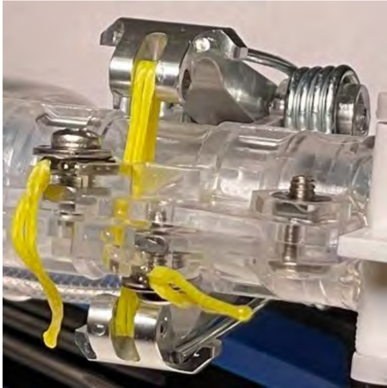
(Internal portion of housing zoomed in on hemostasis valve.)
