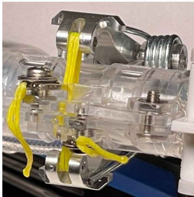
(Image of internal portion of housing zoomed in on hemostasis valve.)
