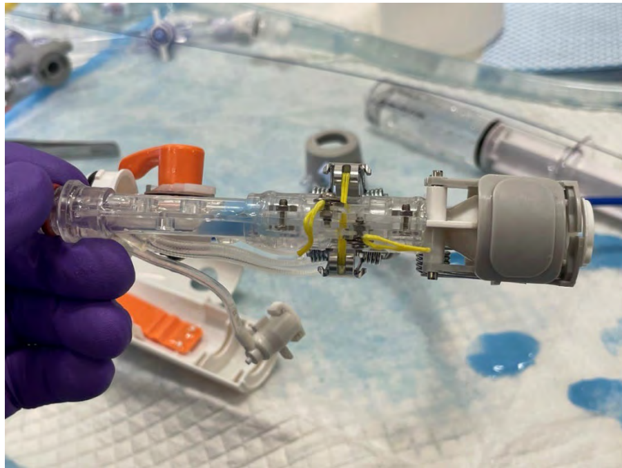
17 (Image of internal portion of housing with hemostasis valve.) 18 19 20 21 22 23 24 25 26 27 28
