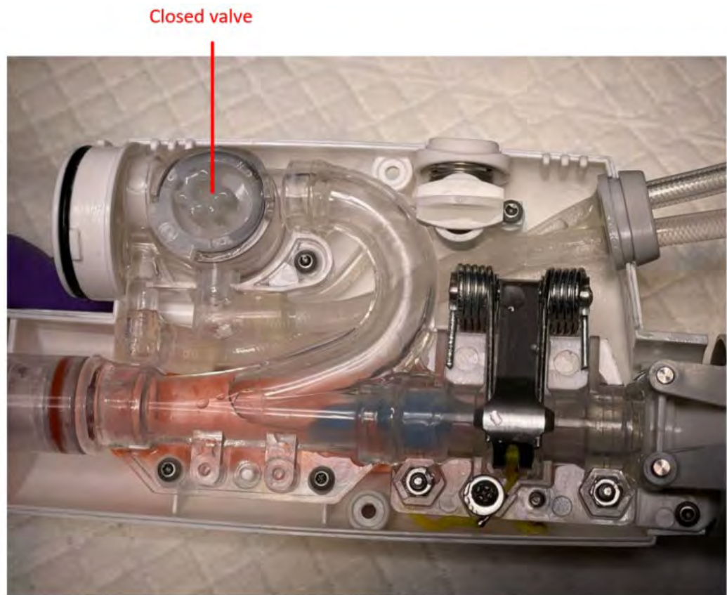
26 (Annotated image of Symphony housing (internal).)
