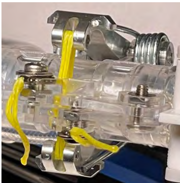
28 (Image of internal portion of housing zoomed in on hemostasis valve.)
