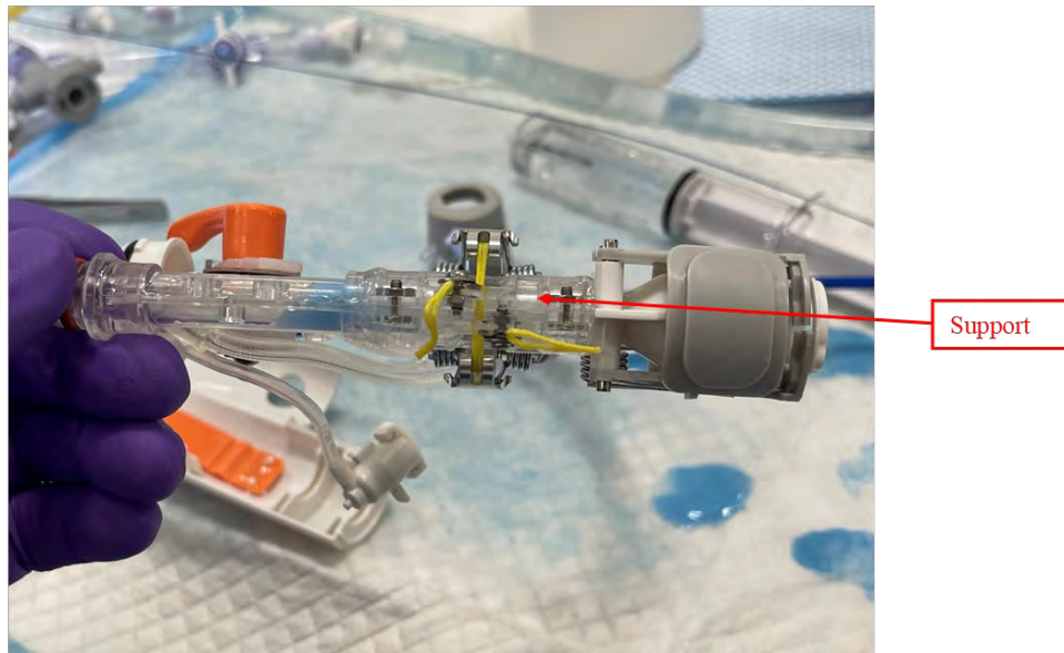
(Image of internal portion of housing with hemostasis valve.)
