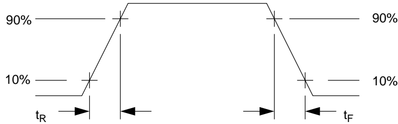
Figure 5A-12 — Signal levels for rise and fall times
